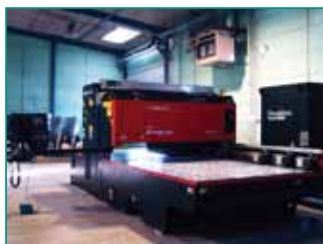
AMADA laserskjærer 4KW 1500x5000x12mm
