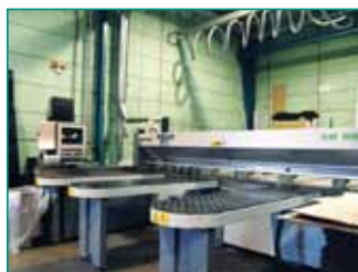
SELCO EB 95mm sag (finér/tre/ plast)3800x3200mx 80mm med optimering
